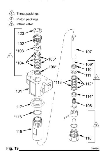
3. Tighten the nut (110) onto the piston valve (108) to 2 in-lb (0.23 N.m). See Fig. 20.
